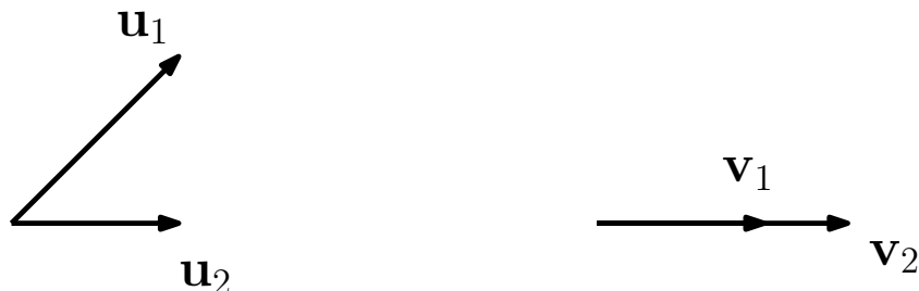
Figure 1: A pair of sets of two vectors in \mathbb{R}^2 . The set \{\mathbf{u}_1, \mathbf{u}_2\} is linearly independent. The set \{\mathbf{v}_1, \mathbf{v}_2\} is linearly dependent; indeed, \mathbf{v}_2 = 1.5\mathbf{v}_1 .
